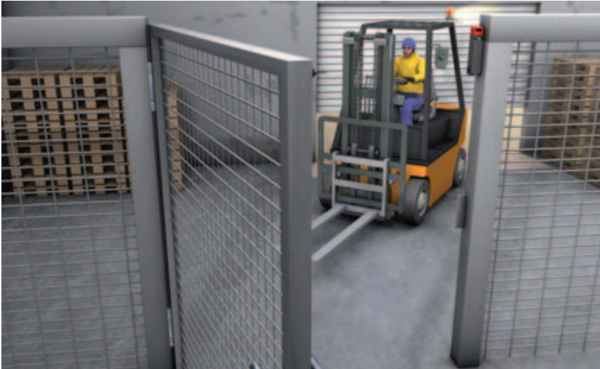
Heavy-Duty L200 Safety Locking Device on a very large gate in a logistics operation with forklift traffic
