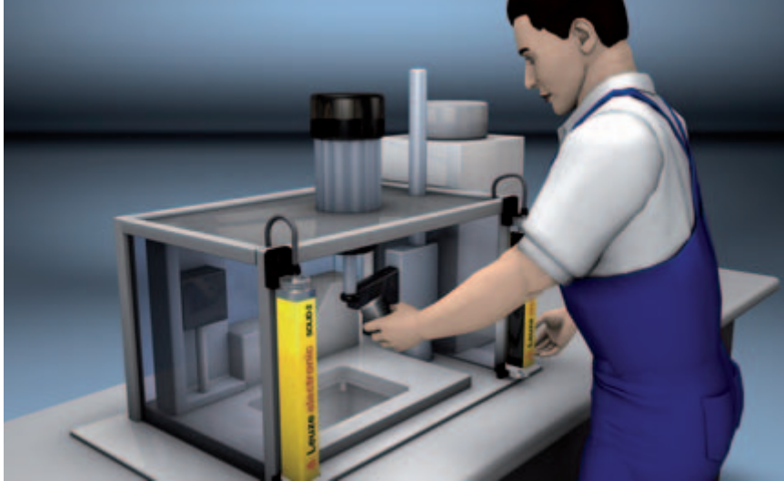
The cycle control function of the configurable MSI Safety Relays allows efficient semi-automatic processes
