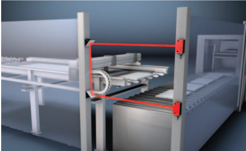
Access guarding with Single Light Beam Safety Devices and US Deflecting Mirrors
