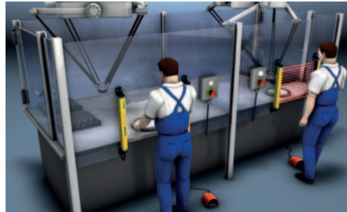
Control of individual safety components with programmable Safety Controllers.
