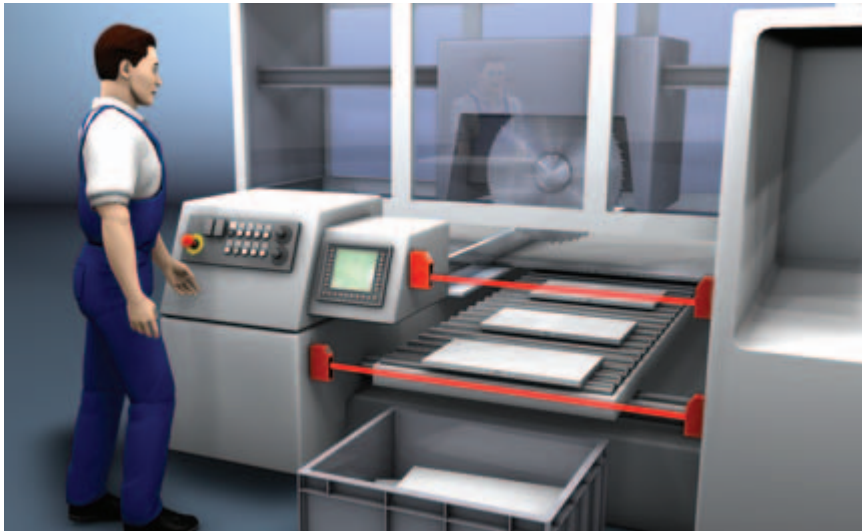
Guarding at a wood processing machine with an SLSR 46B Single Light Beam Safety Device
