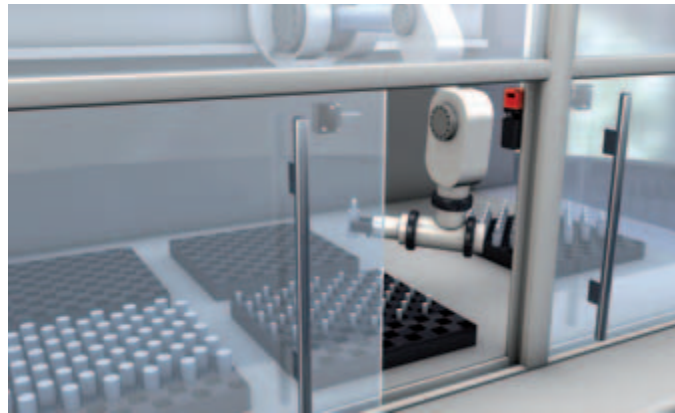
Safety Switch for guarding the sliding door on a pick-and-place machine
