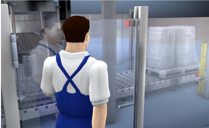
S200 Safety Switch on the door of a plastic film wrapping station
