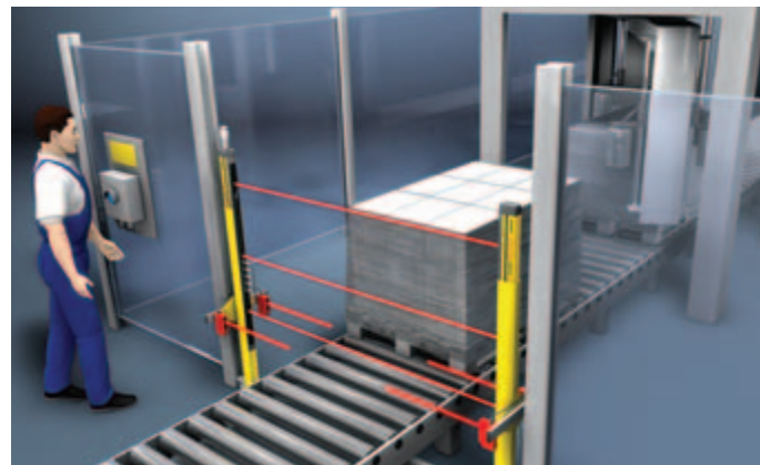
Muting with Safety Sensor Set in a wrapping machine application
